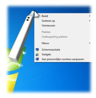
When you press the second button (until the first resistance to have the primary action), the mouse-cursor will jump to the tip of the Vmarker pen. Releasing the button will show the right-click-menu just like with the right-mouse-button.
