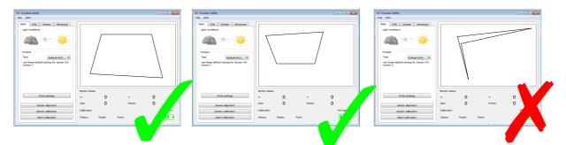
Above you can see different examples; the first, most left, could be the result after calibration of a Vmarker sensor placed on a table. The second could be a ceiling mounted Vmarker sensor, somewhat further away, but acceptable.
